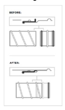
Gasket-Tite is our next generation of self-sealing duct systems at Spiral Pipe of Texas. Available in round sizes from 4" to 48" diameter, we give you the ability to easily assemble duct systems that exceed ASHRAE and energy code leakage standards --- but without the need for mastic sealants.
